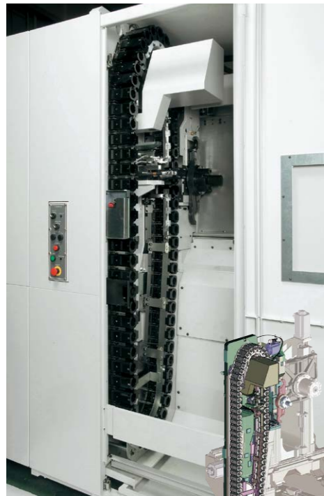
Chain system ATC magazine (64 tool: Optional)
